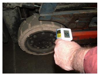
To measure heat in the actual tire, aim infrared digital thermometer at several spots on the tread and sidewall of the tire. Unless there is a wide variance of temperature, record the highest temperature reading.
